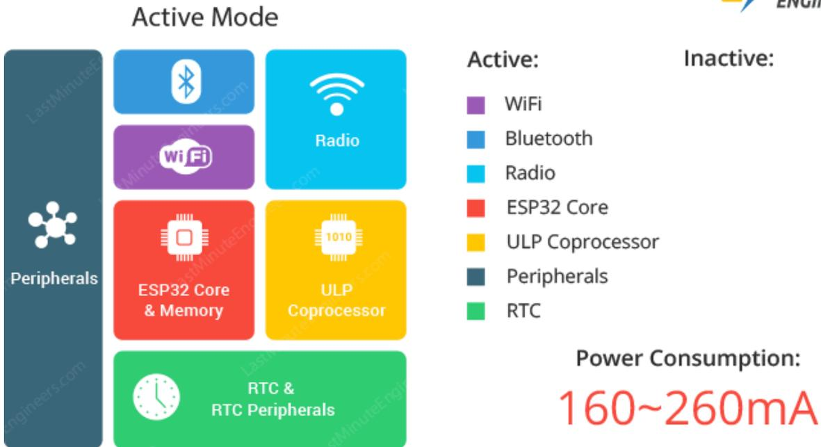
If you look at the ESP32 datasheet, power consumption during Active power mode, with RF working is as follows:
