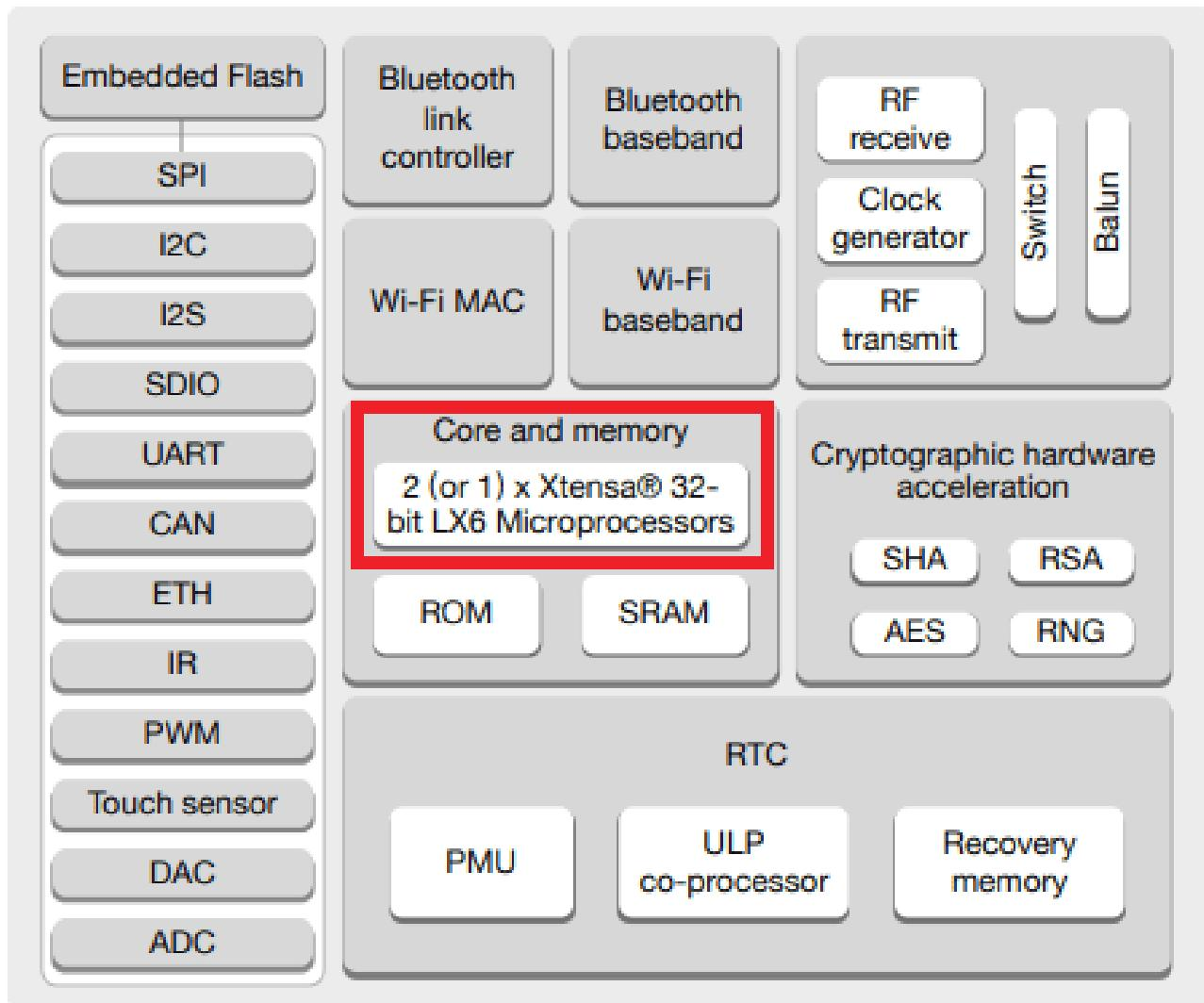
When we upload code to the ESP32 using the Arduino IDE, it just runs – we don't have to worry which core executes the code.
