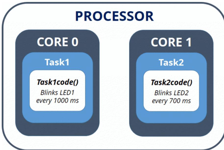
Upload the next sketch to your ESP32 to blink each LED in a different core:
