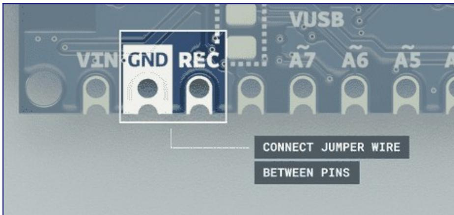
3. When the board is connected, it will open the mass storage device. You can now remove the jumper wire.
