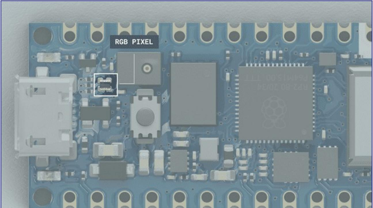
The Nano RP2040 Connect features a built-in RGB that can be utilized as a feedback component for applications. The RGB is connected through the W-102 module, so the WiFiNINA library needs to be installed and included at the top of your sketch to work.
