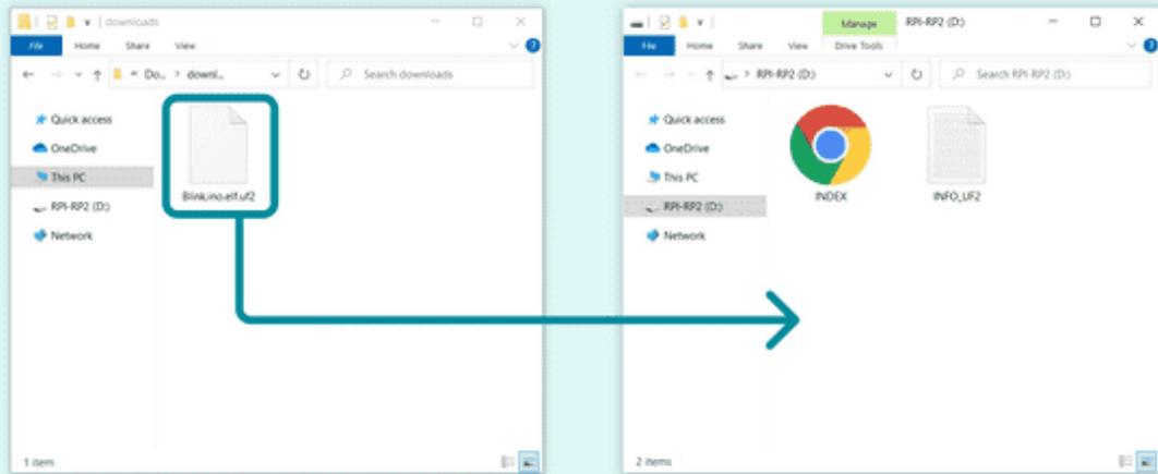
After dragging the U2F file, the board will be flashed with a program that blinks the built-in LED, and shifts between the red, green and blue pixels.
