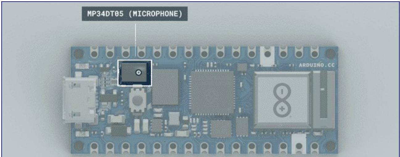
The MP34DT05 is a compact, low-power omnidirectional digital MEMS microphone with an IC interface. It has a 64dB signal-to-noise ratio, is capable of sensing acoustic waves and can operate in temperatures of -40 °C to +85 °C.
