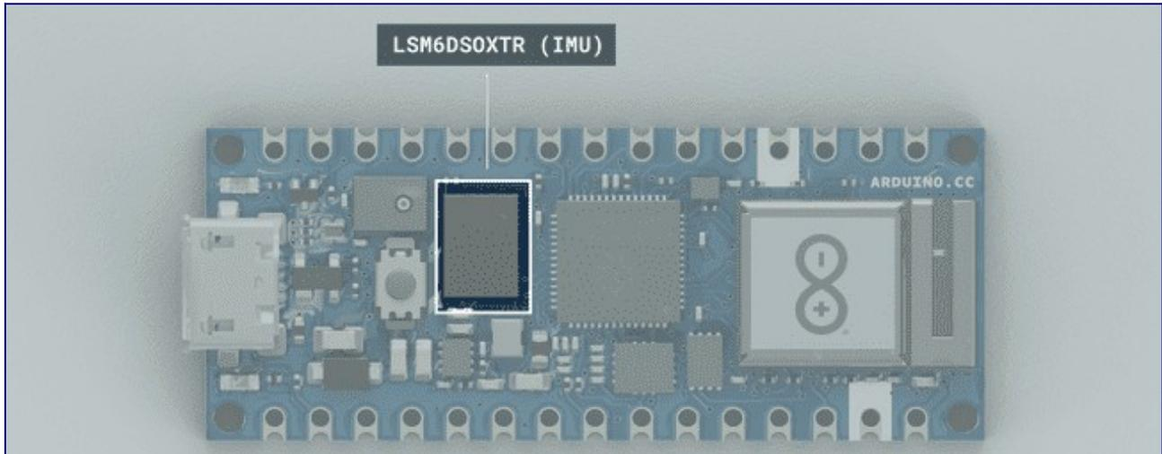
The LSM6DSOXTR from STM is an Inertial Measurement Unit that features a 3D digital accelerometer and a 3D digital gyroscope. It features among many other things, a machine learning core, which is useful for any motion detection projects, such as free fall, step detector, step counter, pedometer.
