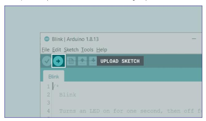
When the code is uploaded, the text "Done uploading." is visible in the bottom left corner. If you look closely at your board, you will notice an orange LED blink with an interval of one second. This means you have successfully uploaded a program to your board.
