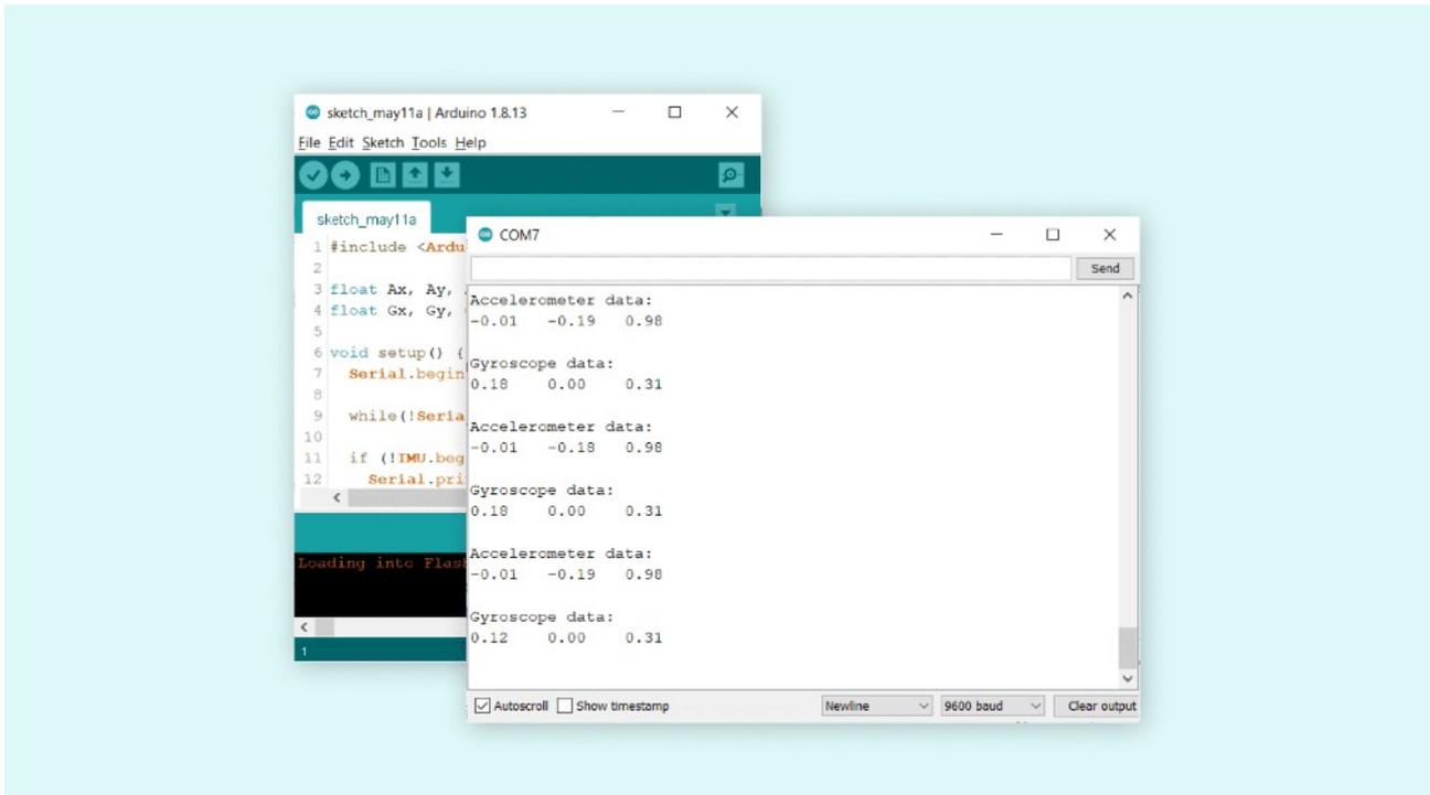
The data is being printed with an interval of 500 milliseconds. This can be adjusted by changing the line `delay(500)` at the bottom of the sketch.
