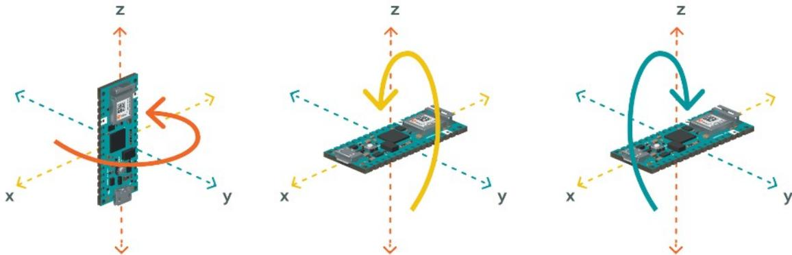
Gyroscope sensors are also called "Angular Rate Sensors" or "Angular Velocity Sensors". Measured in degrees per second, angular velocity is the change in the rotational angle of the object per unit of time.
